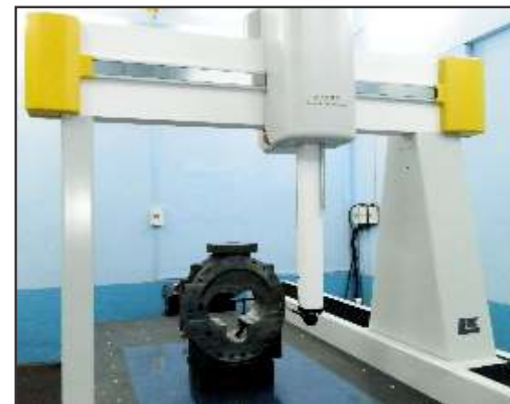
Each Housing is inspected on CMM for ensuring consistency in machining
