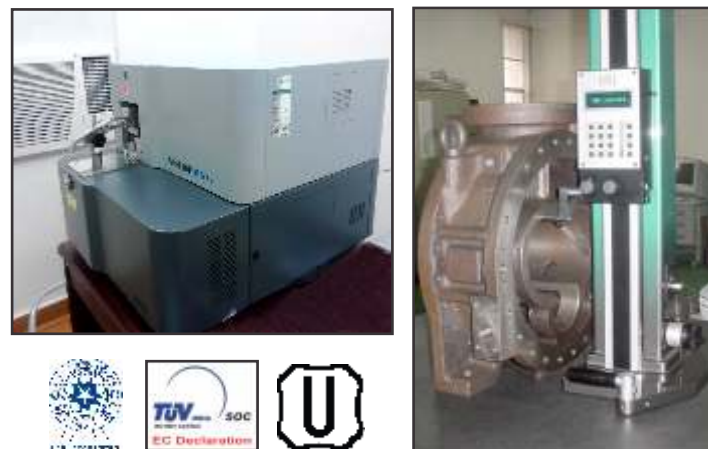
Quality Checking of Machined Equipment by Spectro (NABL Accredited) & Trimos Machine for accuracy
